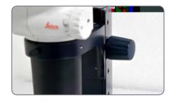
The focusing drive can be operated either left- or right-handed.
