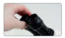
2. Check that the eyepieces are seated firmly and precisely in place.
